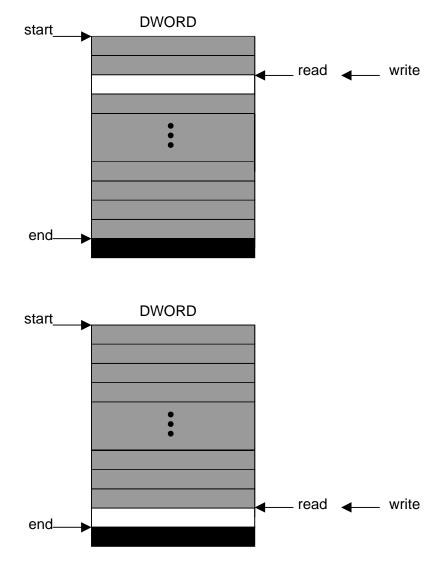
From Figure 8, it can be seen that the physical size of a queue is one dword larger than the number of references in the queue when it is full. Therefore in order to create a queue that holds 128 references, the software must allocate contiguous memory of 129 dwords.
