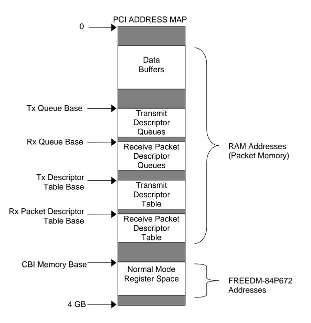
When multiple FREEDM-84P672's are attached to the bus, each FREEDM-84P672 must have a unique set of the following data structures:
