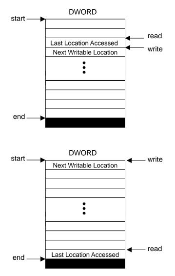
The full queue states are illustrated in Figure 8. The queue is full when the read index is equal to the write index.
