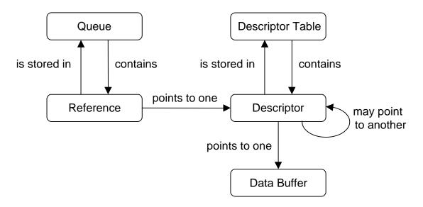
These data structures are also accessed by software. The queues specify the data which may be accessed by the FREEDM-84P672 or the software, but not both simultaneously.
