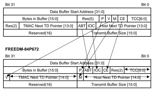
The Transmit Channel Code (TCC) field increased from 7 bits to 10 bits as a result of the increase in addressable HDLC channels from 128 to 672 for the FREEDM-84P672.
