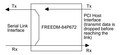
Serial links can be placed in line loopback by setting the appropriate bit within one of the following registers. There are 84 bits corresponding to the 84 serial links.
